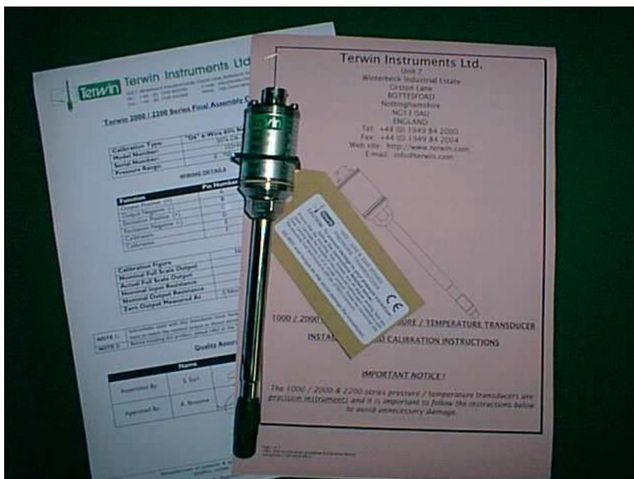
The protective cap and gasket should be left on the transducer until such time that the mounting port on the extruder has been prepared for use using a Transducer Mounting Hole Cleaning Tool Kit. Installation of transducers into ports that are contaminated with old material is one of the primary causes of failure as hardened plastics can tear the diaphragm and this means that the transducer is rendered useless.
